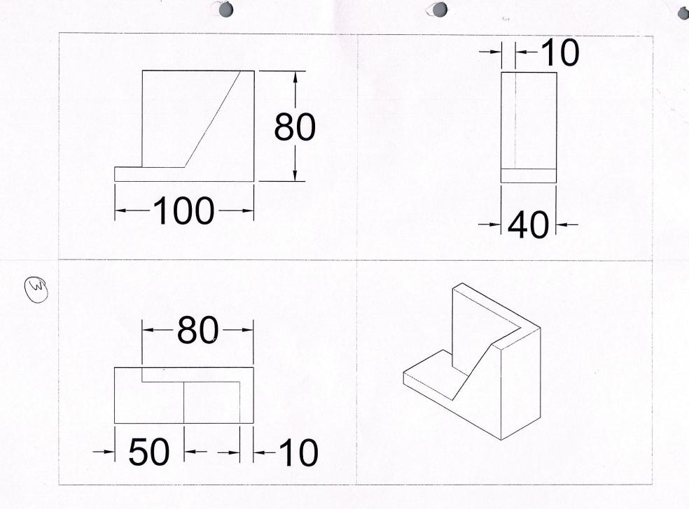
Aim: To Plot Isometric view and Generate orthographic views for a given Diagram
