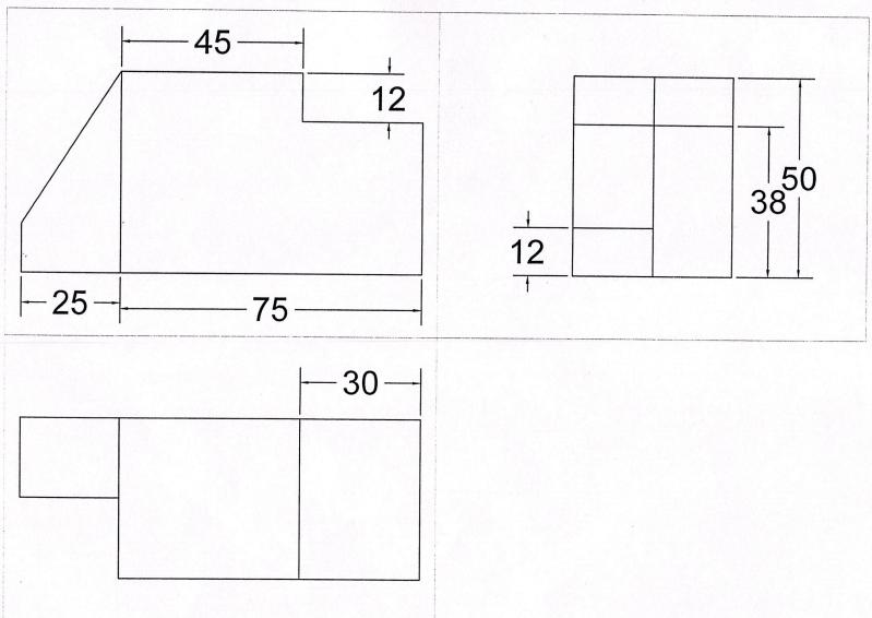
Aim: To Plot Isometric view and Generate orthographic views for a given Diagram
