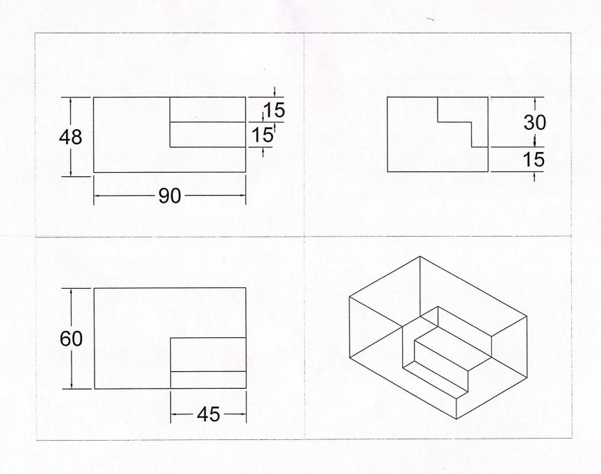
Aim: To Plot Isometric view and Generate orthographic views for a given Diagram
