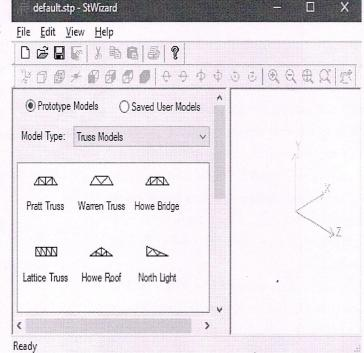
Using the above prototype models we can create simple structures quickly like we can create different trusses as shown in above snapshot. For Instance let us assume we need to create a bay frame then follow below steps:
